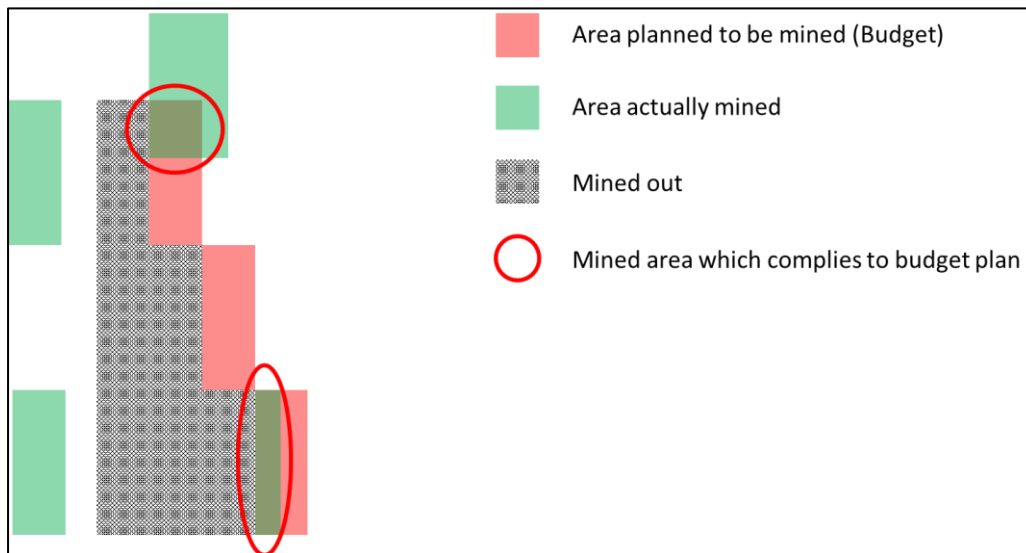
Figure 21: Schematic illustration indicating how the mining compliance with the budget plan for a specific period is calculated.
