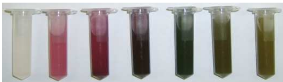
Figure 3.11 Colour change observed after 24h of incubation at 65°C in the presence of varying gold(III) concentrations. F.l.t.r. 0.1; 0.5; 1; 1.5; 5; 7.5 and 10mM.
