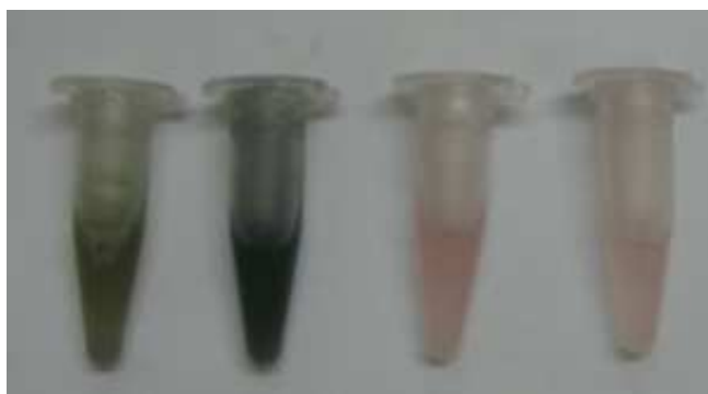
Figure 3.7 Colour change observed after 8h of incubation at 65°C in the presence of 2mM gold(III). F.l.t.r. pH 3.6; pH 5.5; pH 7.5 and pH 9.5.
