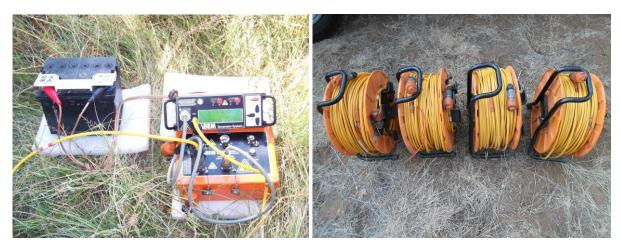
Figure 7-6: Resistivity equipment
