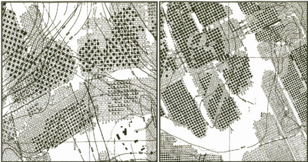
Figure 19. Detailed examples of bord-and-pillar with partial stooping.
