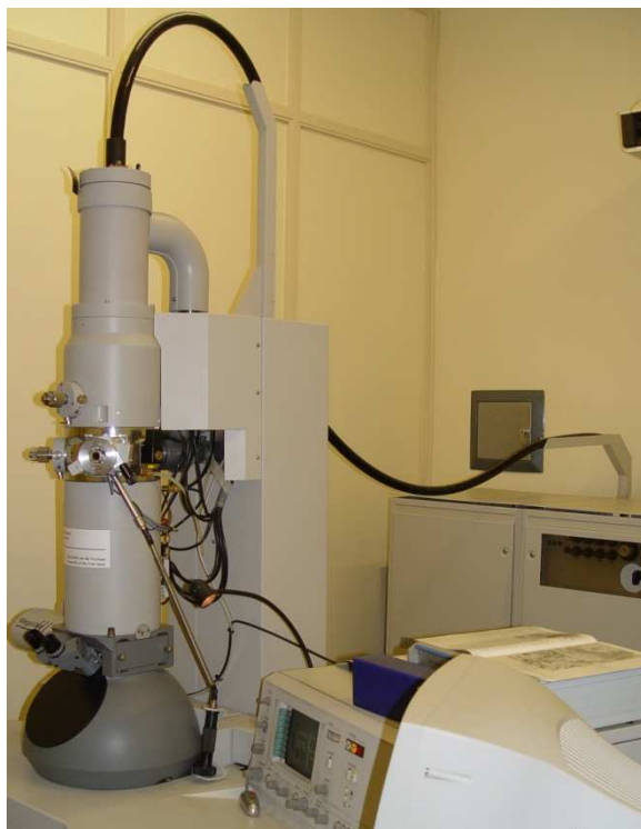
Figure 10: TEM system at the Centre for Microscopy at UFS.
