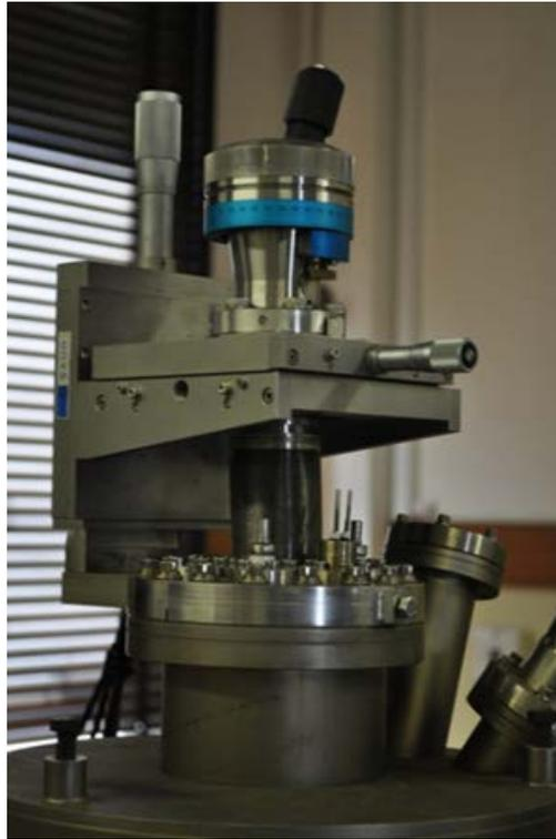
**Figure 5.18:** The fitted manipulator.
