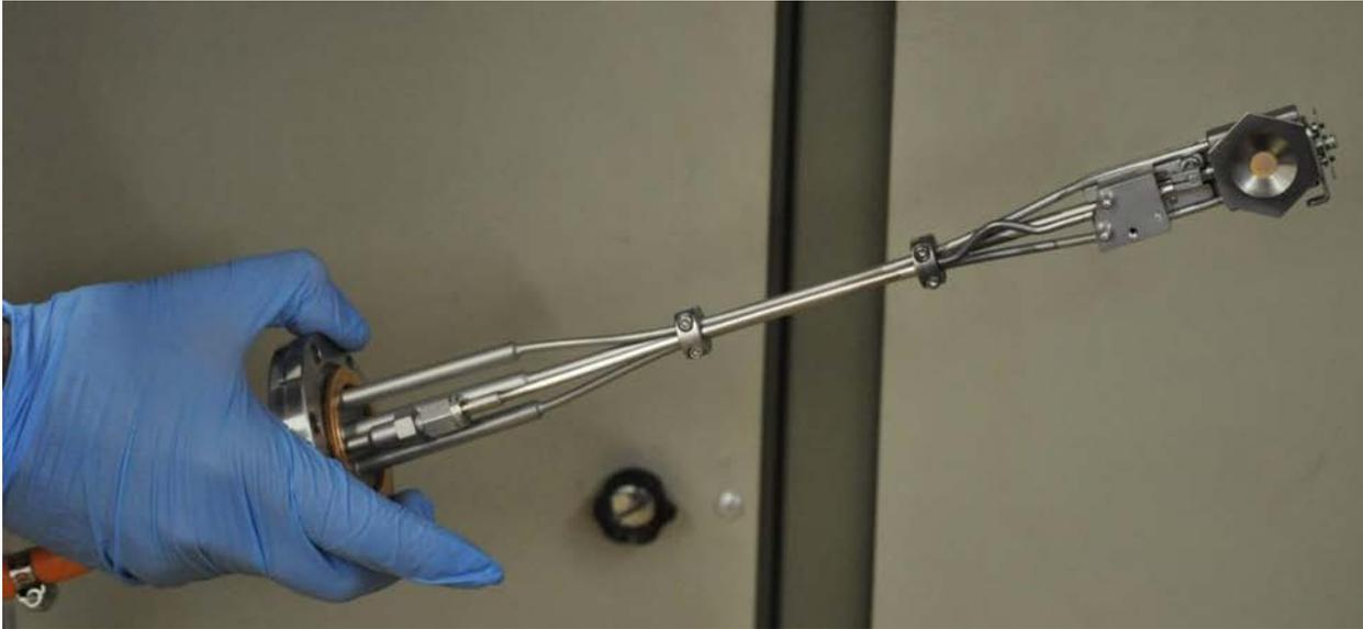
**Figure 5.23:** The deposition monitor arm with water cooling tubing, electrical connections and sensor holder.
