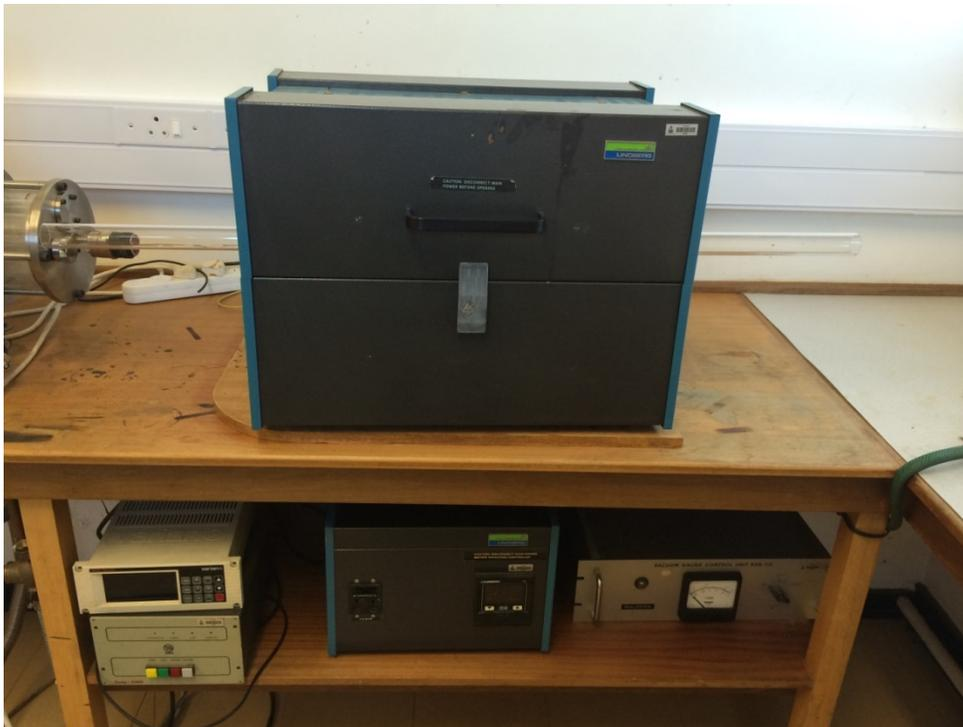
**Figure 5.10:** The Lindberg furnace used during the sample annealing process.
