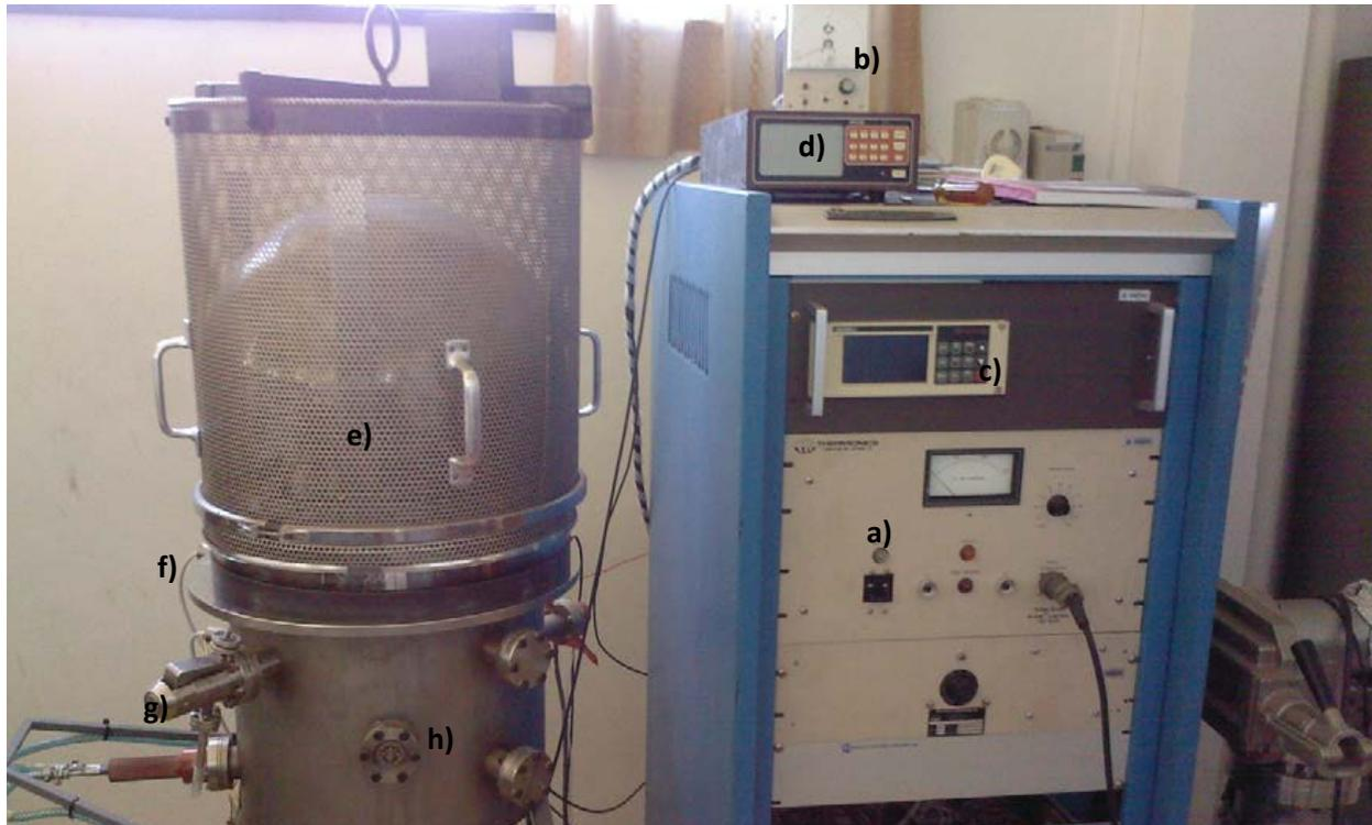
**Figure 5.2:** The evaporation system showing some of the external parts: a) electron gun filament current controller, b) Pirani gauge control unit, c) Varian pressure gauge control unit, d) Inficon thickness monitor, e) glass dome cover, f) High voltage feeds troughs connecting the electron gun filament to the controller, g) linear crucible manipulator, and h) stainless steel vacuum chamber. Not visible on photo: turbo molecular and rotary vane pump system. Adapted from (Joubert, 2010).
