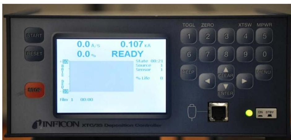
**Figure 5.22:** Inficon XTC/3s Deposition Controller unit
