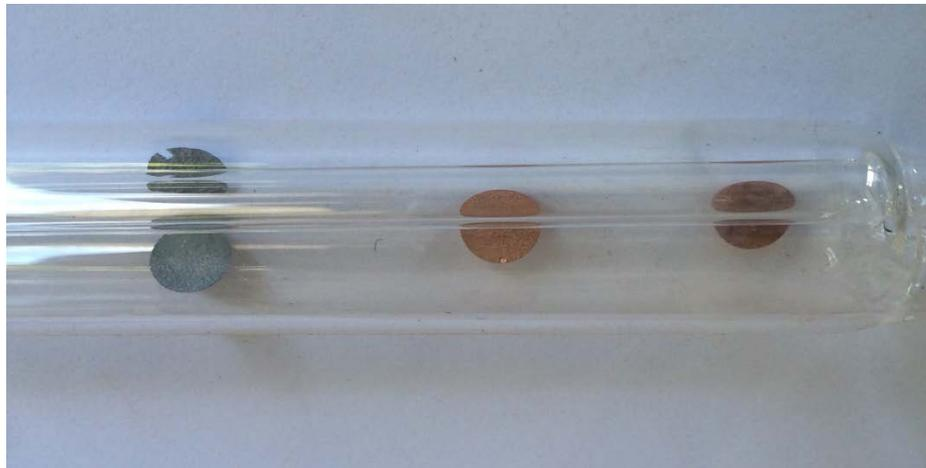
**Figure 5.13:** Failed sample preparation. The antimony did not adhere to the copper crystal.
