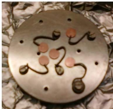
**Figure 5.4:** Cu crystals mounted on a sample plate.
