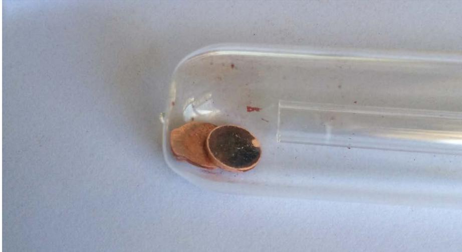
**Figure 5.14:** Failed sample preparation showing possible oxidation of samples.
