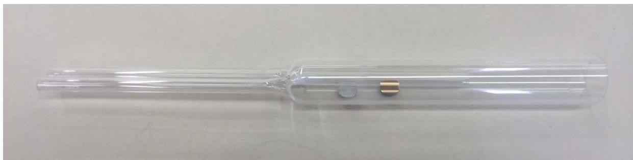
**Figure 5.8:** Quartz tube with samples ready to be sealed.
