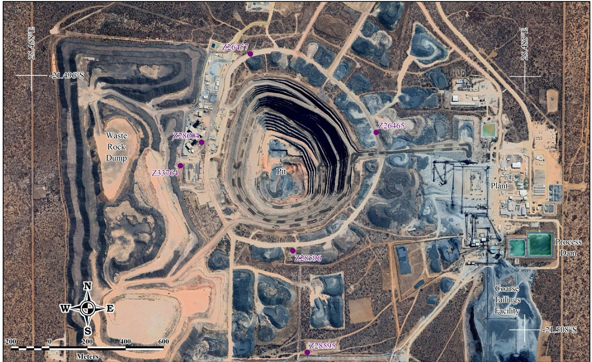
Figure 4.17: Positions of the six boreholes drilled into the Mea-arkose and the weathered granite.
