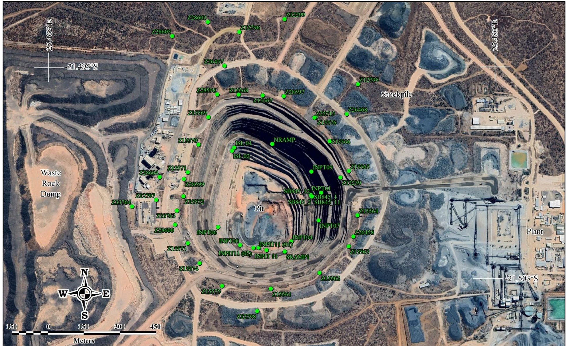
Figure 4.4: Positions of the dewatering boreholes at KDM.
