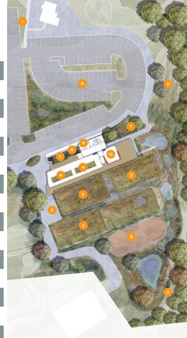
SITE PLAN 1 SEPTIC TANKS (below grade): In this first treatment step, the majority of suspended solids settle out of the water. Naturally occurring microbial organisms living in the water work to digest the sludge that settles to the bottom of the tanks and the now partially clarified water is skimmed off into the Anaerobic Tank. 2 ANAEROBIC TANK (below grade): Here further settling and a process known as anaerobic digestion occurs. 3 CONSTRUCTED WETLANDS: Here the water flows through the root structure of wetland plants. The plants remove nitrates and reduce the Biological Oxygen Demand (BOD - a measure of the rate at which biological organisms use up the available oxygen) and suspended solids in the water. 4 AERATED LAGOONS: In this step, additional wetland plants are suspended in an Aerated Lagoon. In a symbiotic relationship, the plant roots act as a habitat for microbial populations that further scrub the water. 5 SAND FILTER: This stage is the final "polishing" of the water prior to being reintroduced to the environment. Microorganisms living on and between the grains of sand are fed by any remaining organic compounds in the water. 6 SUBSURFACE DISPERSAL (below the parking): At this stage the water is reintroduced to the soil via a subsurface network of chambers. The chambers are "flooded" with the processed water and allowed to percolate into the soil. 7 RAIN GARDENS: Water shed from the building roof is temporarily detained here during a rain shower while plants work to cleanse the water of contaminants before it enters the Rainwater Cistern or is absorbed into the soil. 8 RAINWATER CISTERN: Water is stored here before being used for toilet flushing and other nonpotable uses at the OCSL. 9 MECHANICAL AND ELECTRICAL ROOM: This is the location of inverters for the PV system, rainwater system, and equipment for the eco-machine. Supporting the pedagogical nature of the project, windows between this room and the Lobby expose the inner workings of the building systems. 10 LEARNING LAB: Part of the classroom, this area provides a place for visiting students (everyone is a student here) to perform tests and experiments on the water. 11 WOODLANDS RESTORATION: Future projects will restore the woodlands surrounding the OCSL and elsewhere on campus to their natural state.
