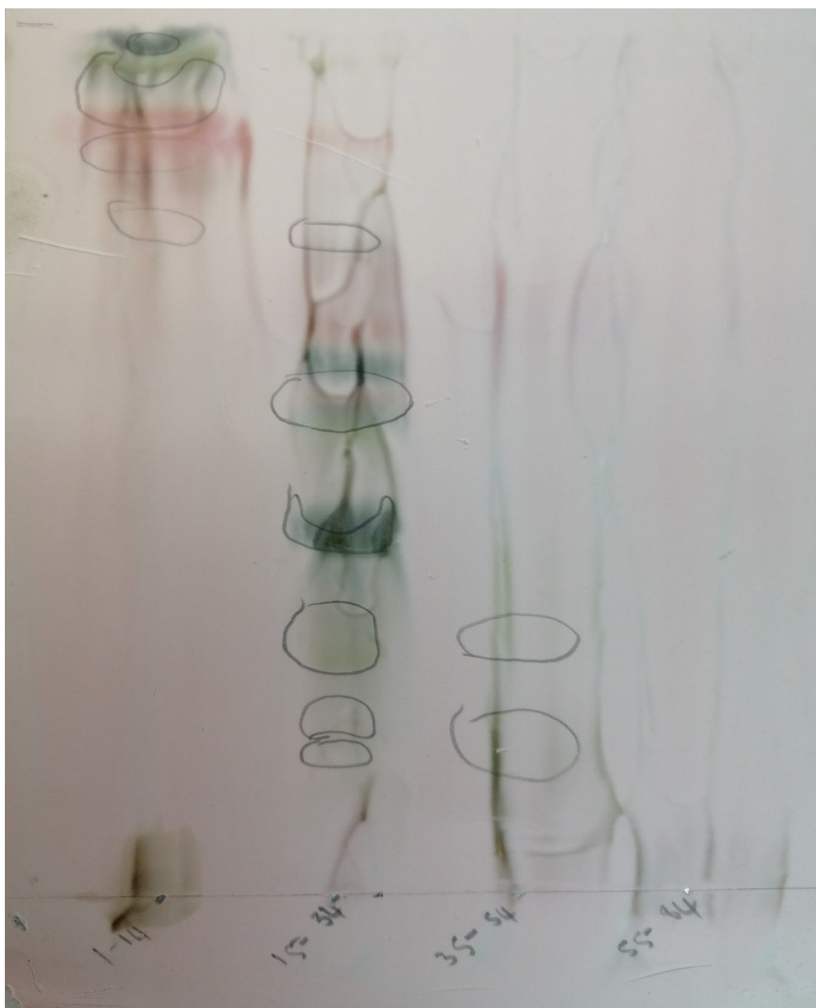
Figure 8.4: After being sprayed with anisaldehyde reagent, the n-hexane combined fractions from the column chromatography were spotted on a TLC plate and developed with n-hexane: ethyl acetate (8:2) solvent system.
