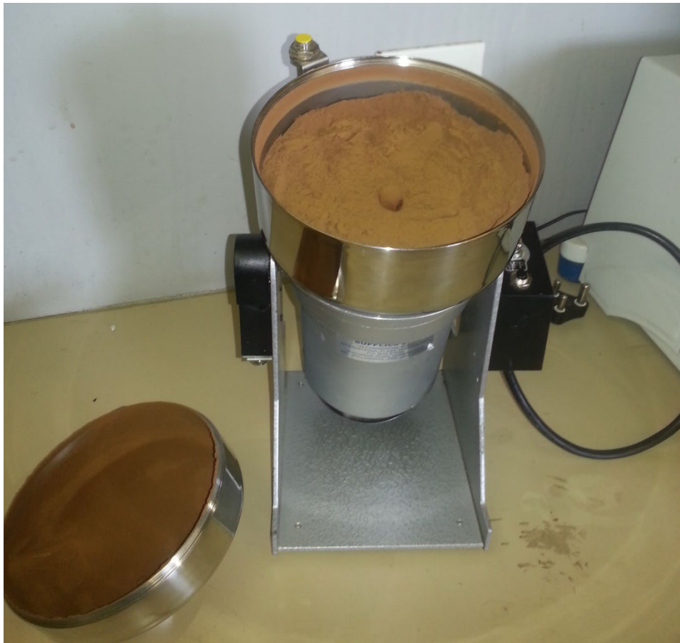
Fig 3.1: A blender was used to turn dried plants into a fine powder.
