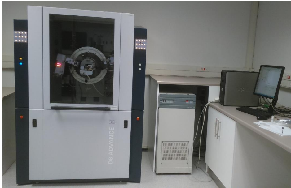
Figure 3.4: The Bruker D8 Advance X-ray diffractometer at the Department of Physics of the University of the Free State.
