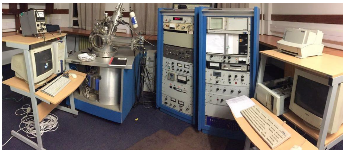
Figure 3.13: PHI Model 549 AES unit at the Department of Physics, University of the Free State.
