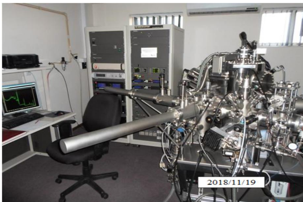
Figure 3.20: PHI 5000 Versaprobe XPS system at the Department of Physics, University of the Free State.
