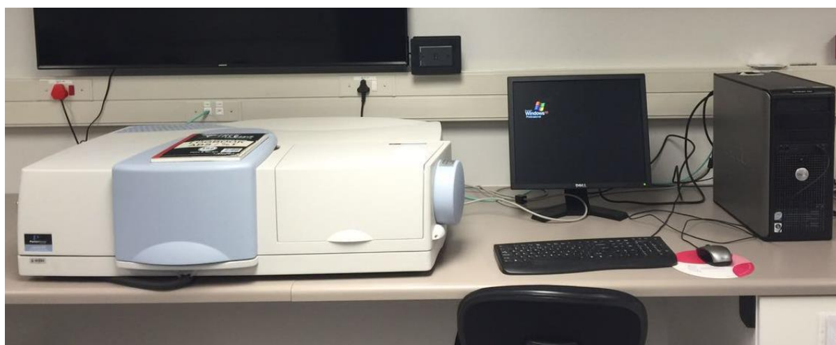
Figure 3.9: PerkinElmer Lambda 950 UV-Vis-IR spectrophotometer at the Department of Physics, University of the Free State.
