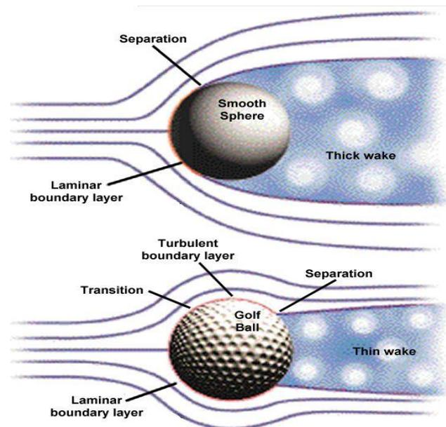
FIGURE 2.5: THE FLOW SEPARATION ON A SPHERE WITH A LAMINAR VERSUS TURBULENT BOUNDARY LAYER (SCOTT, 2005)
