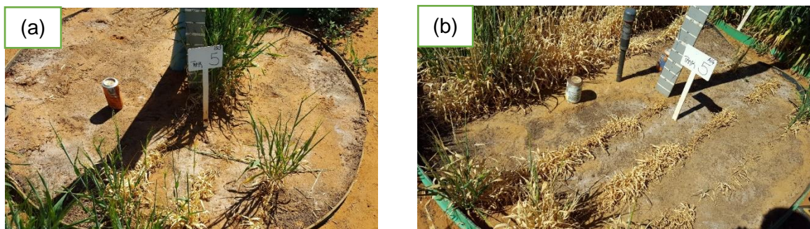
Figure 3.5: Salt precipitation indicated by white patches on the (a) Bainsvlei and (b) Clovelly soil lysimeters irrigated with water of 1200\ mS\ m^{-1} during the second season.
