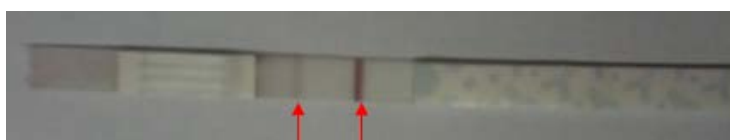
Figure 5.7 Dip strip result when CLB-Pro 35 was used as the capture antibody and VWF/VWFpp polyclonal antibody was used as the detection antibody.
