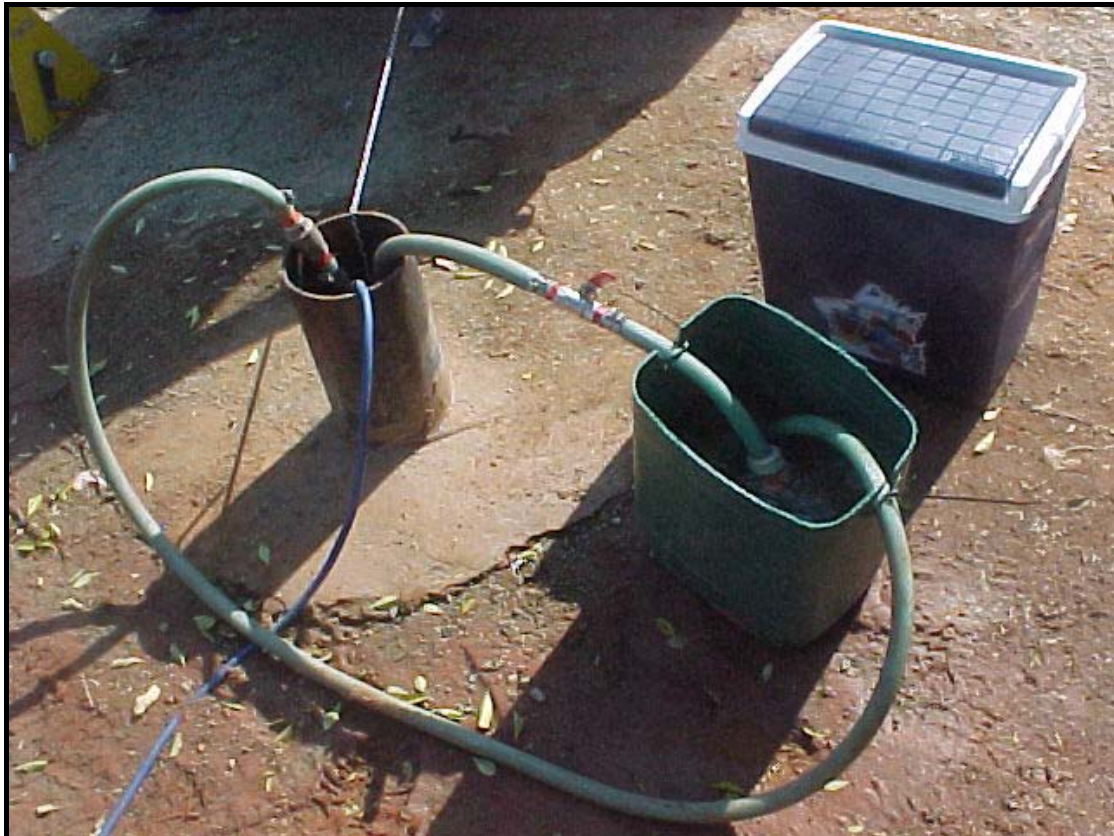
Figure 33: Photo illustrating the arrangement used to conduct the Tracer tests at the Vaalharts
