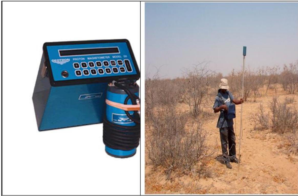
Figure 5-1: The G5 Proton Magnetometer on the left side and the field investigation using magnetometer on the right side.
