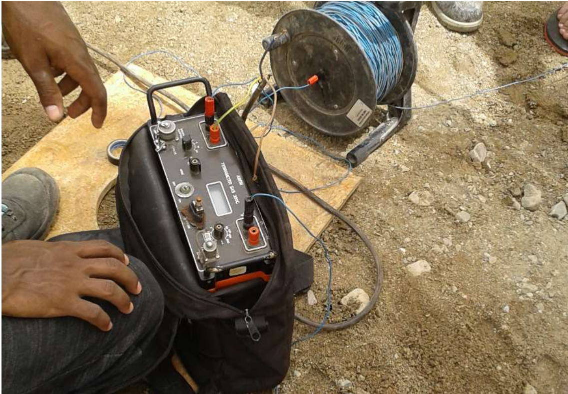
Figure 5-4 Receiver unit used for downhole electrical logging.
