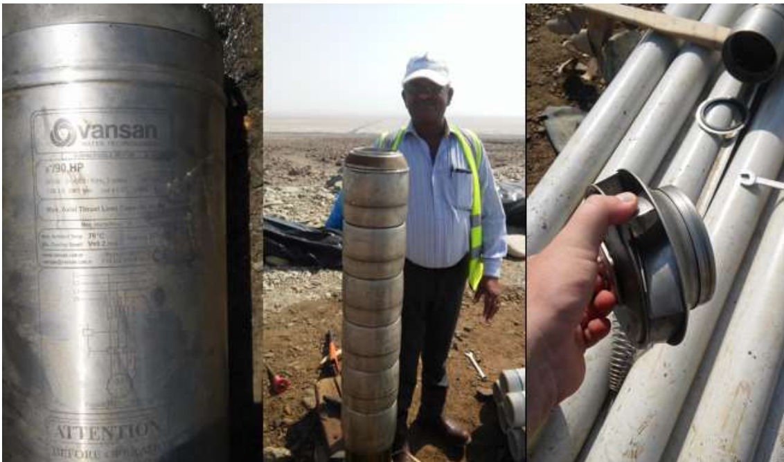
Figure 6-3 Photograph of the Vansan pumps installed at AY-P01, BS-P01, DN-P01 and RAJ-2 respectively, a 6-stage pump and a stainless-steel impeller that was removed.
