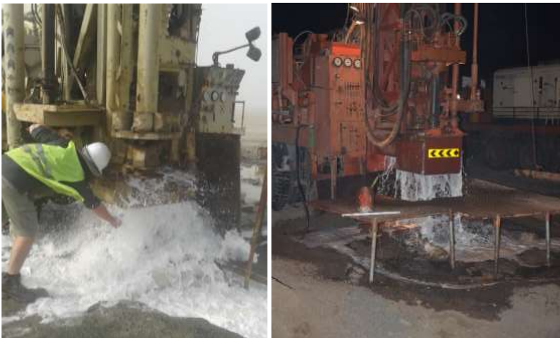
Figure 5-6 Hydrochemical sampling carried out during borehole development.
