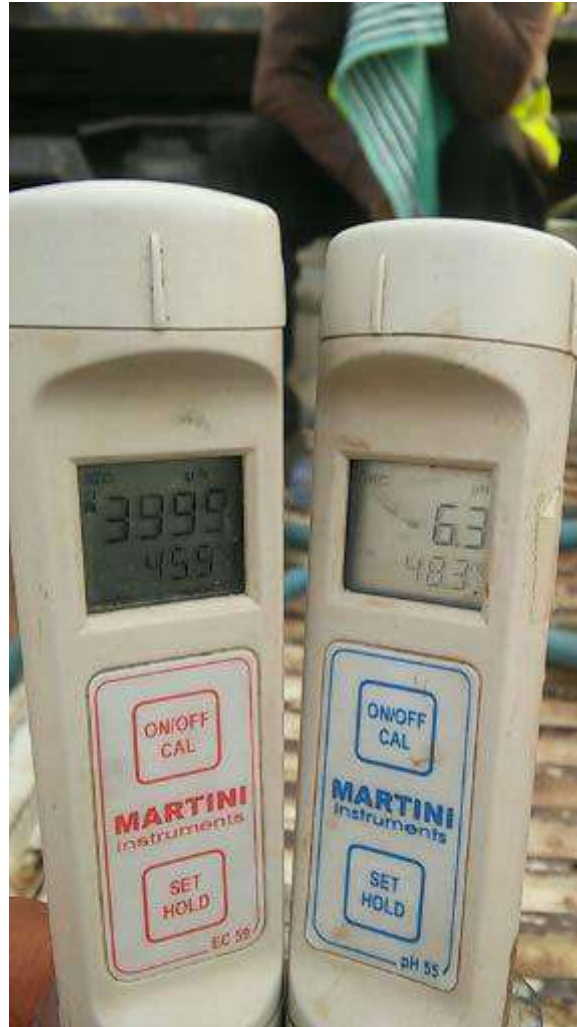
Figure 5-17 Hand held EC and pH meters used to measure water quality in the field after development.
