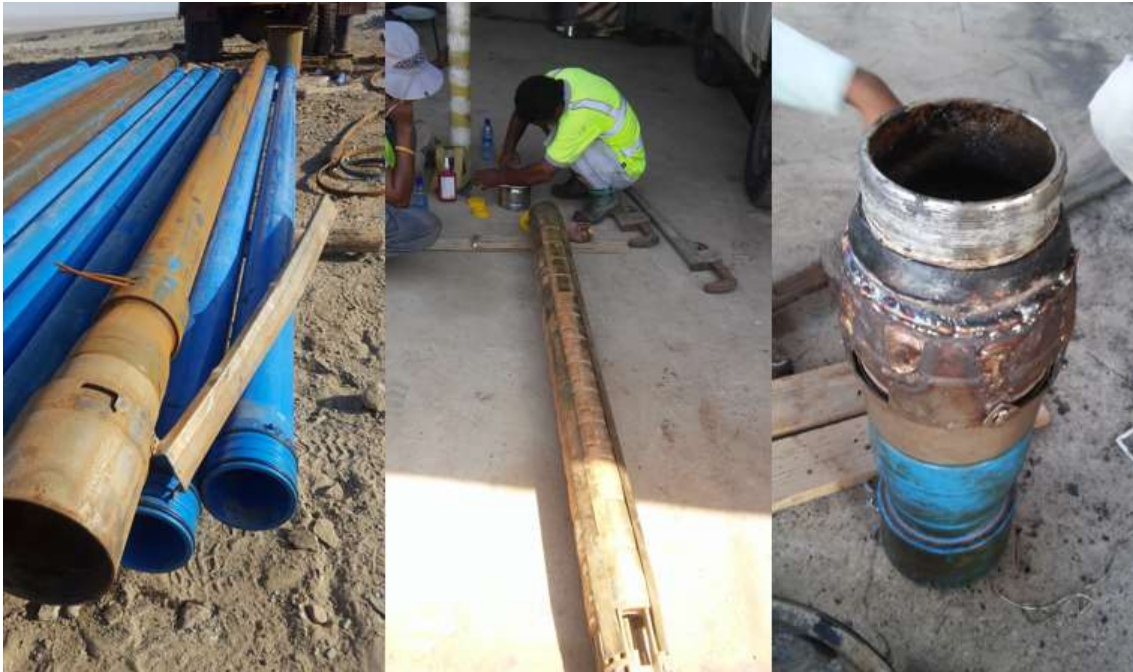
Figure 6-6 Photographs of the RAJ-1 pump housing that broke and resulted in the pump falling down the well, the 13-satge pump and the modified coupling fabricated for the rental pump.
