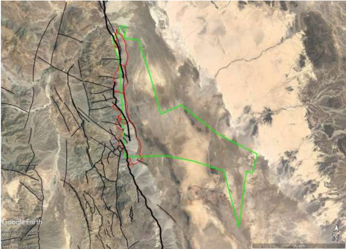
Figure 3-32 Fault and fracture mapping carried out using Google Earth with smaller structures near the concession verified in the field. The thick, black roughly north-south trending line represents the MDRF.
