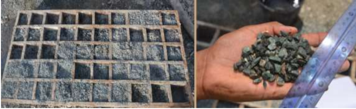
Figure 5-3 Manual logging of drill rock chips in 1 metre intervals.
