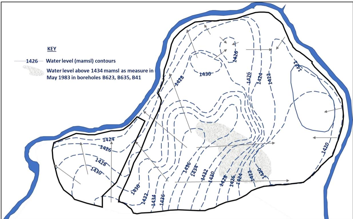
Figure 2.24: Groundwater flow at New Vaal pre- opencast mining (Orpen and Wiegmans, 1983).
