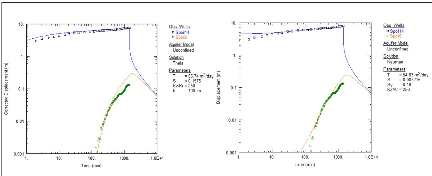
Figure 2.29: Diagnostic plots and hydraulic characteristics for Spoil 14 and Spoil 6.
