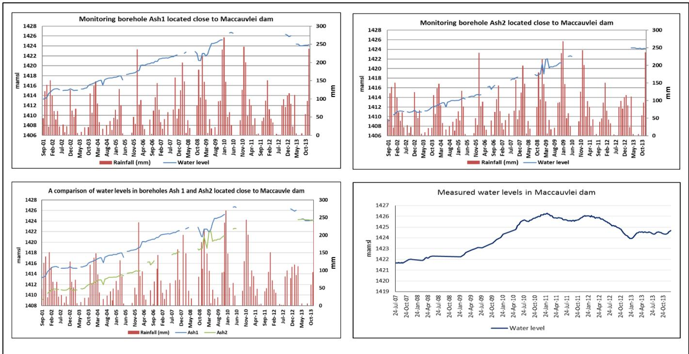
Figure 2.13: Monitoring boreholes in close proximity to the Maccaulei dam and the ash dump
