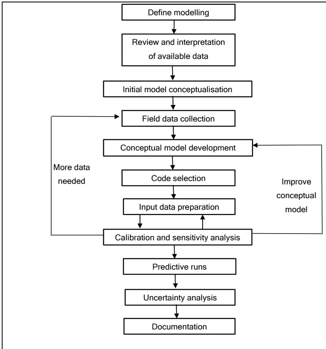
Figure 2.1: An illustration of the iterative nature of groundwater modelling (Bear *et al.*, 1992)
