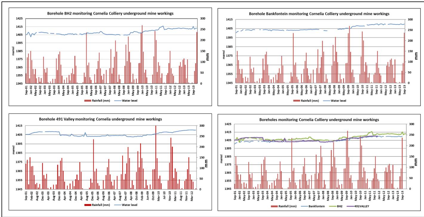
Figure 2.18: Monitoring boreholes targeting Cornelia Colliery's underground mine voids.
