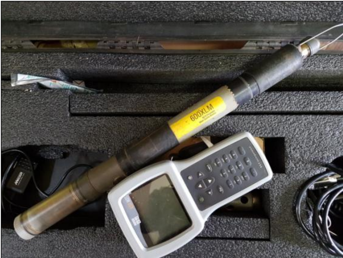
Figure 4.10 YSI (Yellow Spring Incorporated) 600XLM Sonde multi-parameter in-situ monitoring apparatus.
