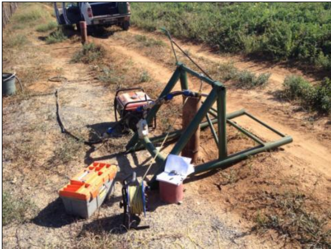
Figure 4.12 Pumping rig and equipment used during pumping tests.
