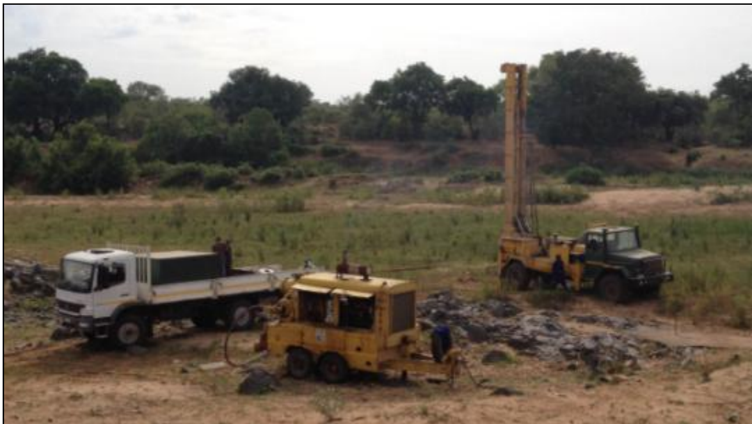
Appendix A-2: The drilling rig is a modified old 10 ton 6x6 SAMIL truck with a super rock 5000 air percussion rig and a 900CFM compressor.
