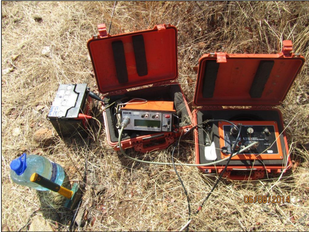
Appendix A-1: ABEM Terrameter that was used for the geophysical survey (Strydom, 2014).
