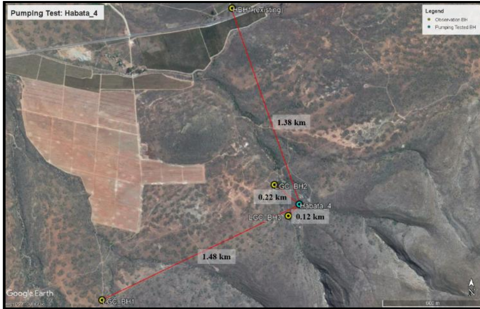
Figure 50: Pumping test at Habata_4 and distribution of observation boreholes.
