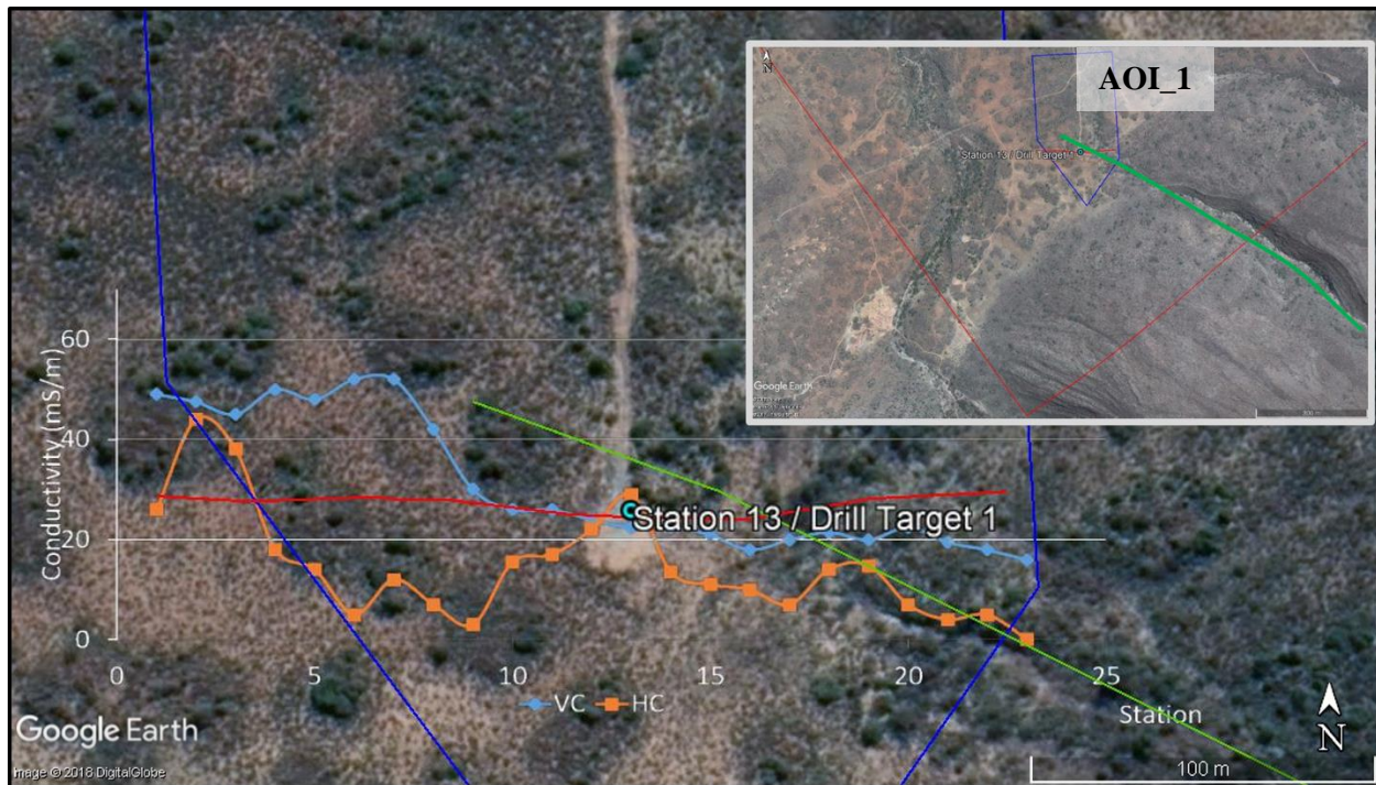
Figure 8: EMP_1 traverse (red line) with shallow (light blue) and deep (orange) measurements, as well as the location of Drill Target 1 at Station 13. The green lineament represents the primary fracture targeted.
