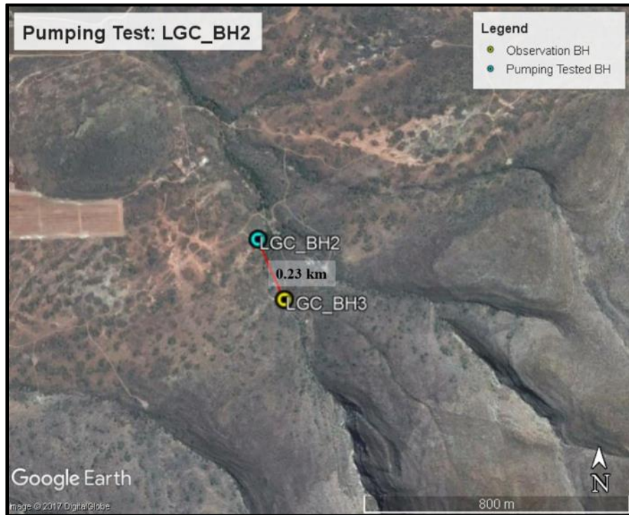
Figure 25: Pumping test at LGC_BH2 and distribution of observation boreholes.
