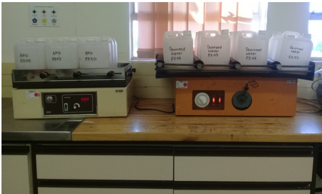
Figure 3.40: Experimental setup for determining the attenuation effect of soils on AMD pollution
