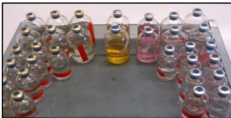
Figure 3.5: Anaerobic serum vials containing enrichment media. Left: PSGM, Middle: two vials containing yeast extract and Right: ASRM.
