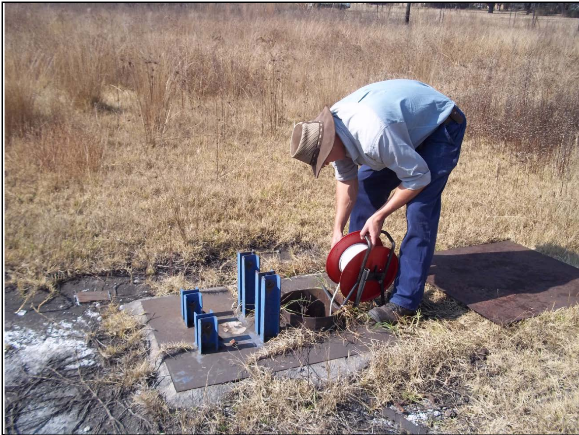
Figure 5-1: Groundwater level measurement with an electronic dip meter in the field.
