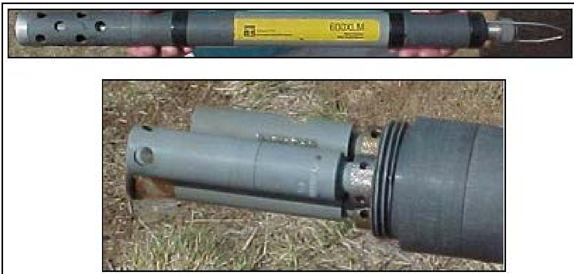
Figure 5-2: Multi-parameter probe with different sensors.
