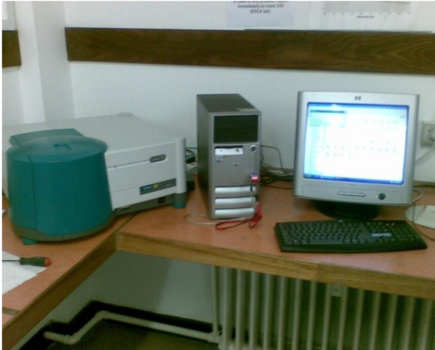
Figure 2.4: Cary Eclipse Photoluminescence Spectrophotometer equipped with a 150 W xenon lamp as the excitation source
