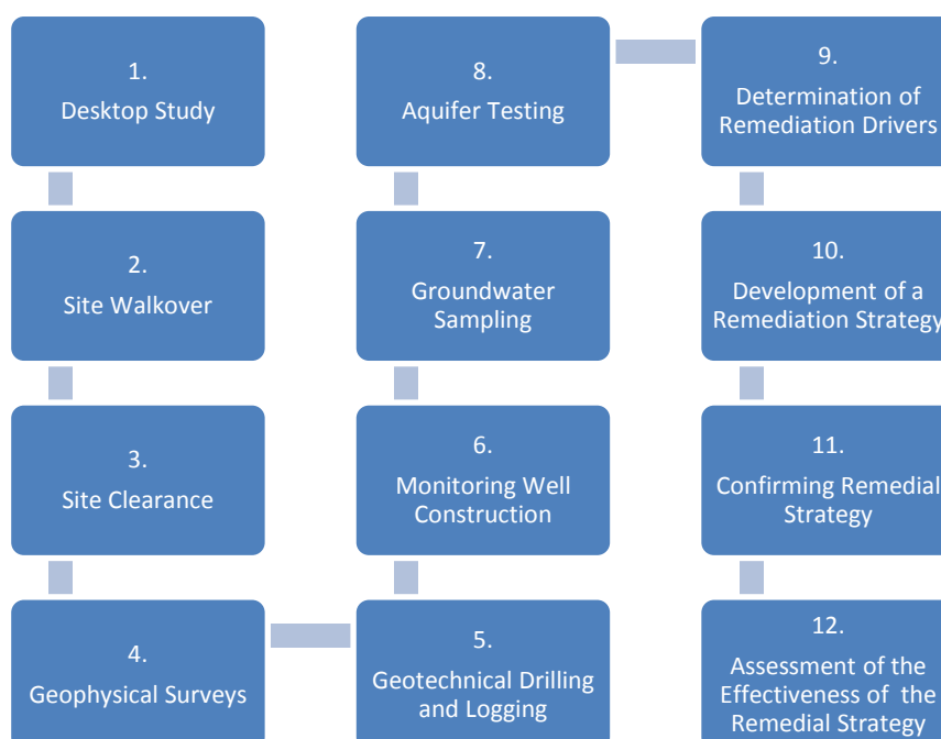
Figure 8-1: Twelve Step Guide to Detailed Site Investigation for Groundwater Contamination within Fractured Aquifers
