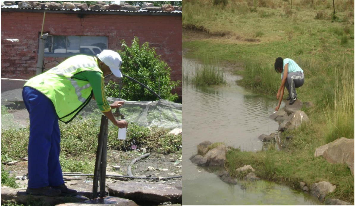
Figure 7-2: Sampling for ground and surface water samples
