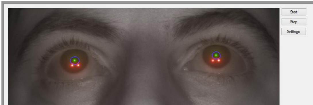
Figure A.10 - Correctly calibrated exposure, gain and gamma
