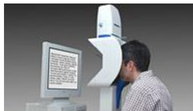
Figure 2.9 - A tower-mounted eye tracker from Sensoric Motor Instruments Source: http://www.smivision.com/uploads/tx_templavoila/iviewx_hi_speed.jpg Retrieved on: 12/06/2014
