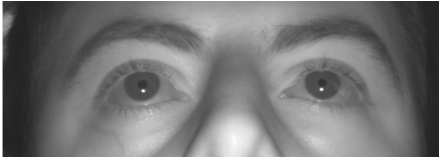
Figure 2.10 – A frame from a typical eye video with a single IR light source
