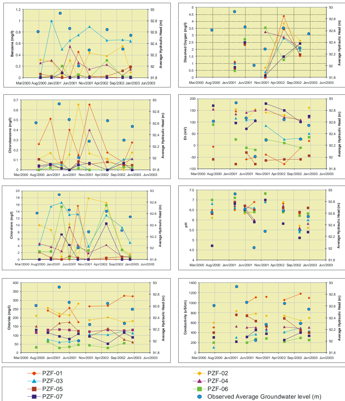
Figure 4.17 - Time series graphics of the most relevant contamination and biodegradation parameters.
