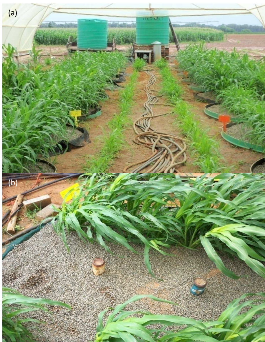
Figure 2.6 (a) Pearl millet cultivated in the two rows of drainage lysimeters under the moveable rain shelter (b) view of top of lysimeter tank with surface covered with quartz gravel illustrating two neutron probes pipes per tank and pearl millet stand.
