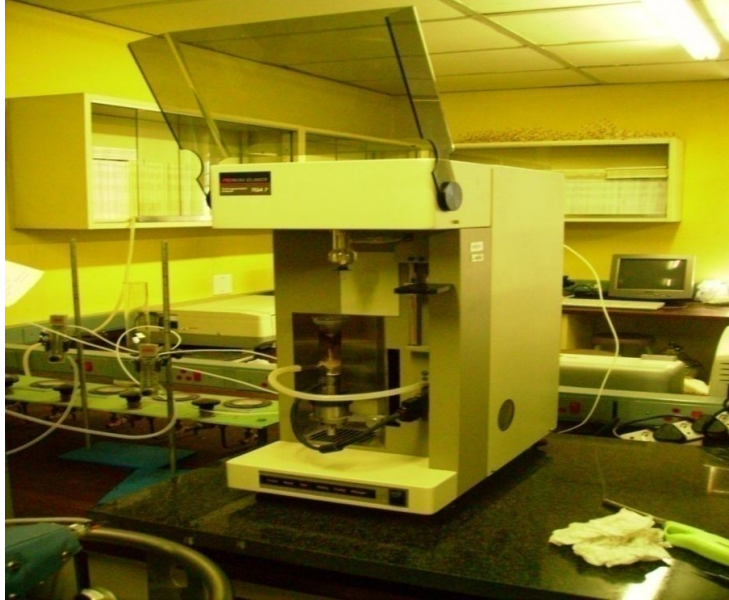
Figure 4.8(b): Image of the TGA apparatus used in this project
