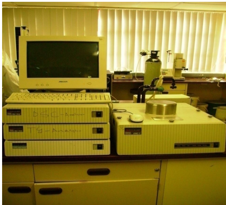
Figure 4.7(d): The Perkin-Elmer DSC7 thermal analyzer used in this study
