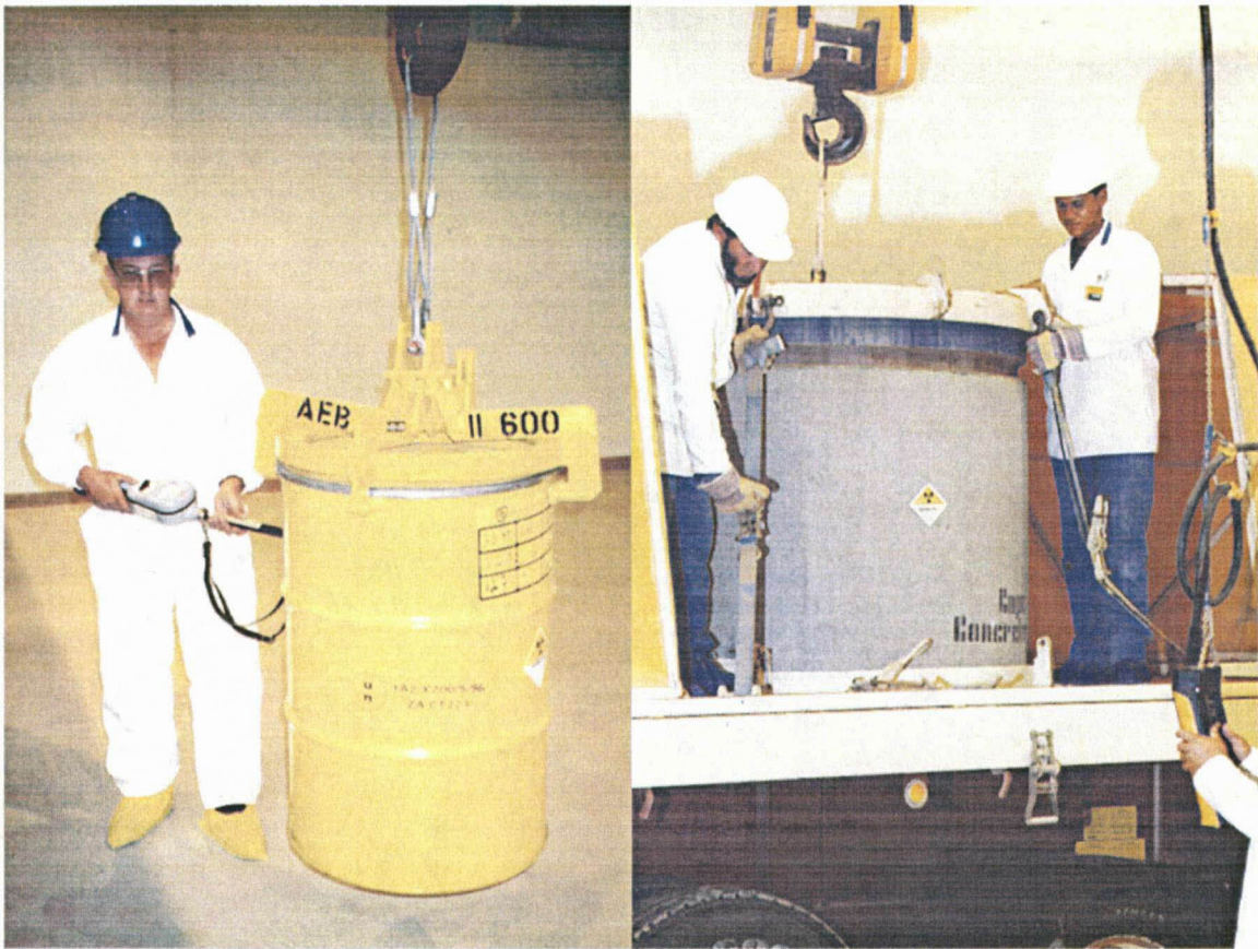
Figure 5-3 The waste packages used for the disposal of radioactive waste at Vaalputs.
