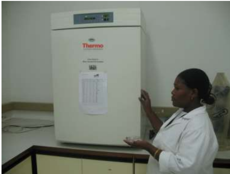
Plate 3.6 Thermo incubator used for in vitro maturation (IVM) and in vitro culture (IVC) of bovine oocytes and embryos respectively
