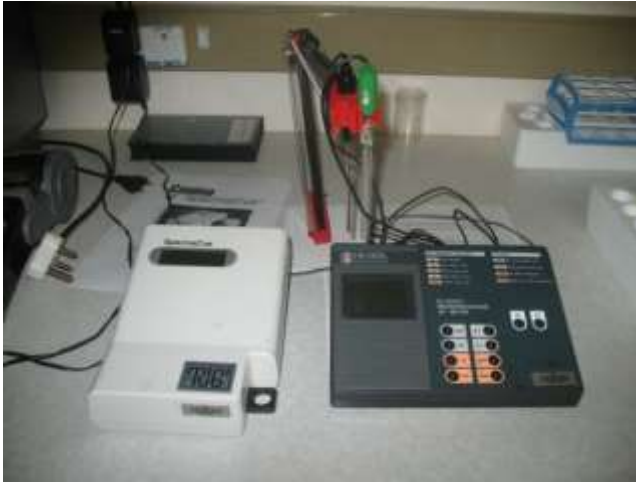
Plate 3.2 Left) Spermacue Photometer for determining sperm concentration in bulls Right) pH meter for measuring pH of the bovine semen samples
