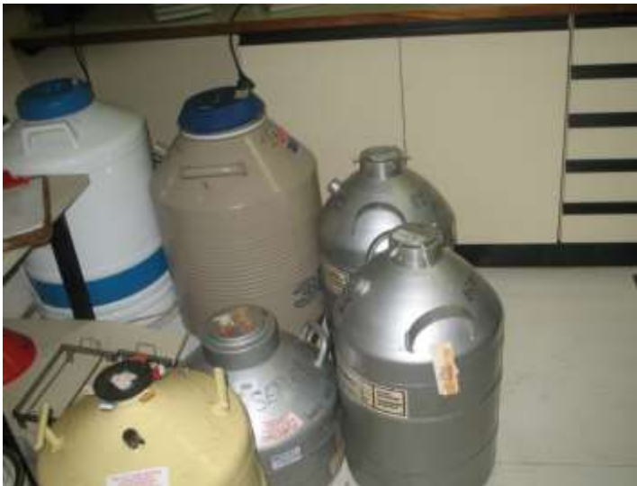
Plate 3.5 Liquid nitrogen tanks for the storage of cryopreserved bovine semen
