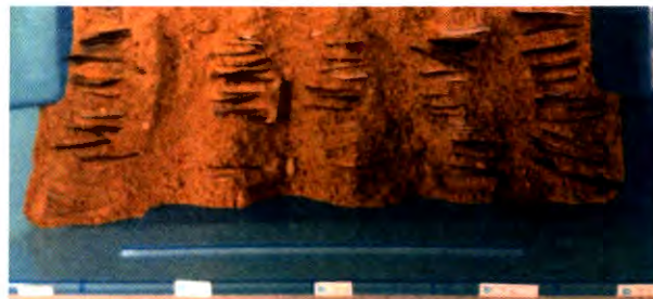
Figure 2.1 The positioning of composite samples in soil for the underground ageing test before covering with soil
