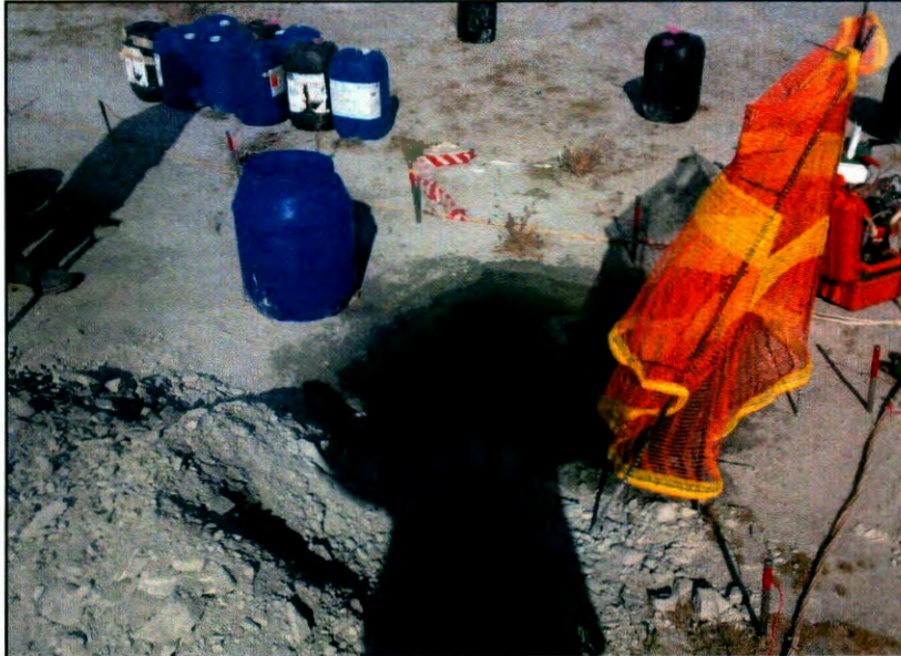
Figure 3.7 Photograph of the survey setup (view towards the south-east). A constant head level with the ash surface is maintained in the injection pit during the injection phase.
