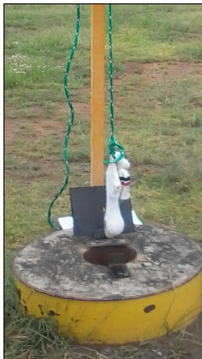
Figure 4-5 Salt was introduced into the injection borehole using an injection sock which was tied to a rope. The sock was slowly lowered down and up the borehole so that significant change in the salinity of the groundwater throughout the borehole was created.
