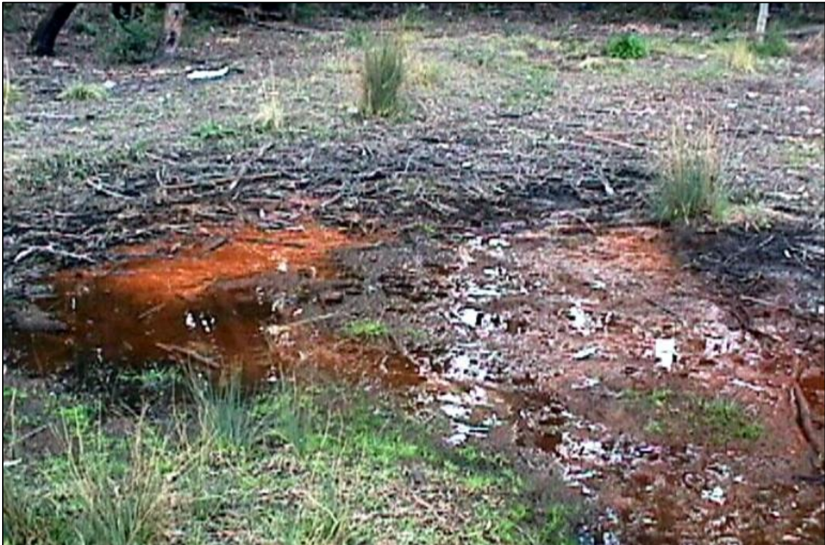
Figure 4: Precipitation of a yellow boy at a South African Colliery (Usher (2003))
