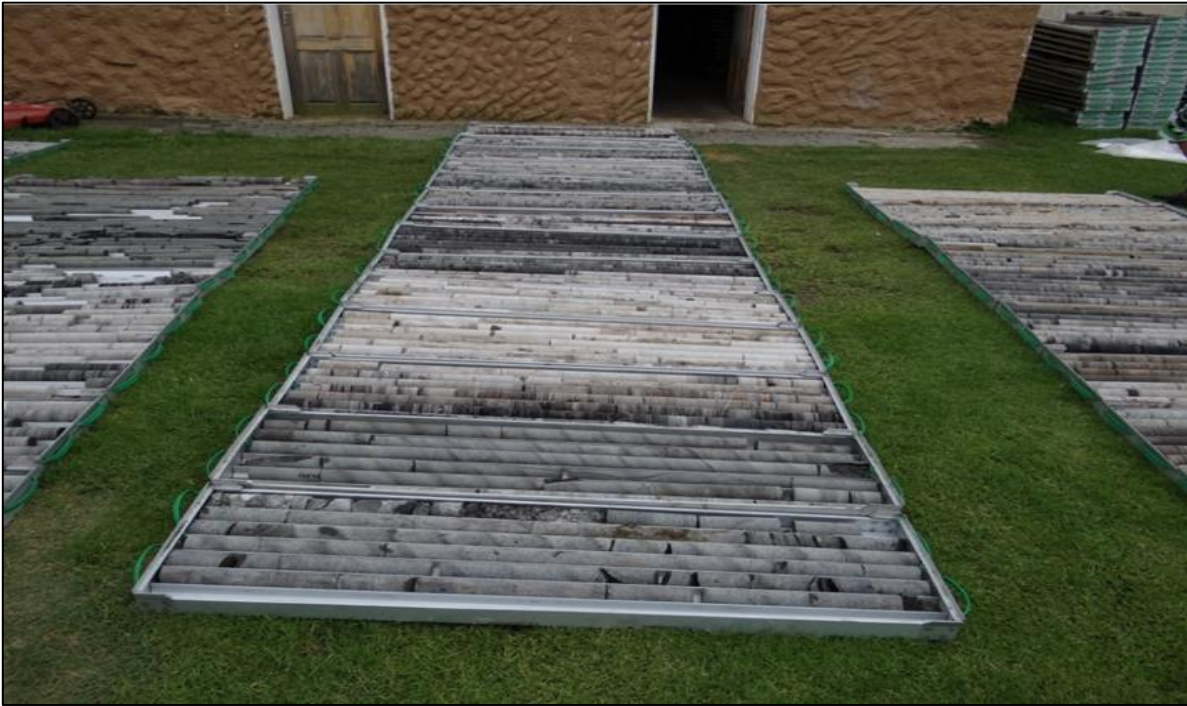
Figure 5: Mine 1 and Mine 2 Borehole core logs
