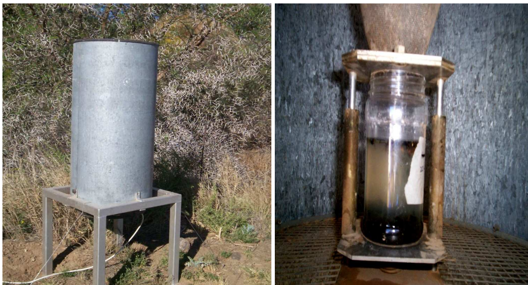
Figure 5. Suction trap with cylinder funnel (left) and the plastic sample bottle with 70% ethanol and glycerol (right) (Photo: J. Adendorff, 2009).
