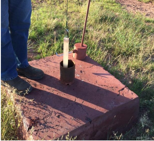
Figure 30a&b: Bailing of water sample at open borehole
