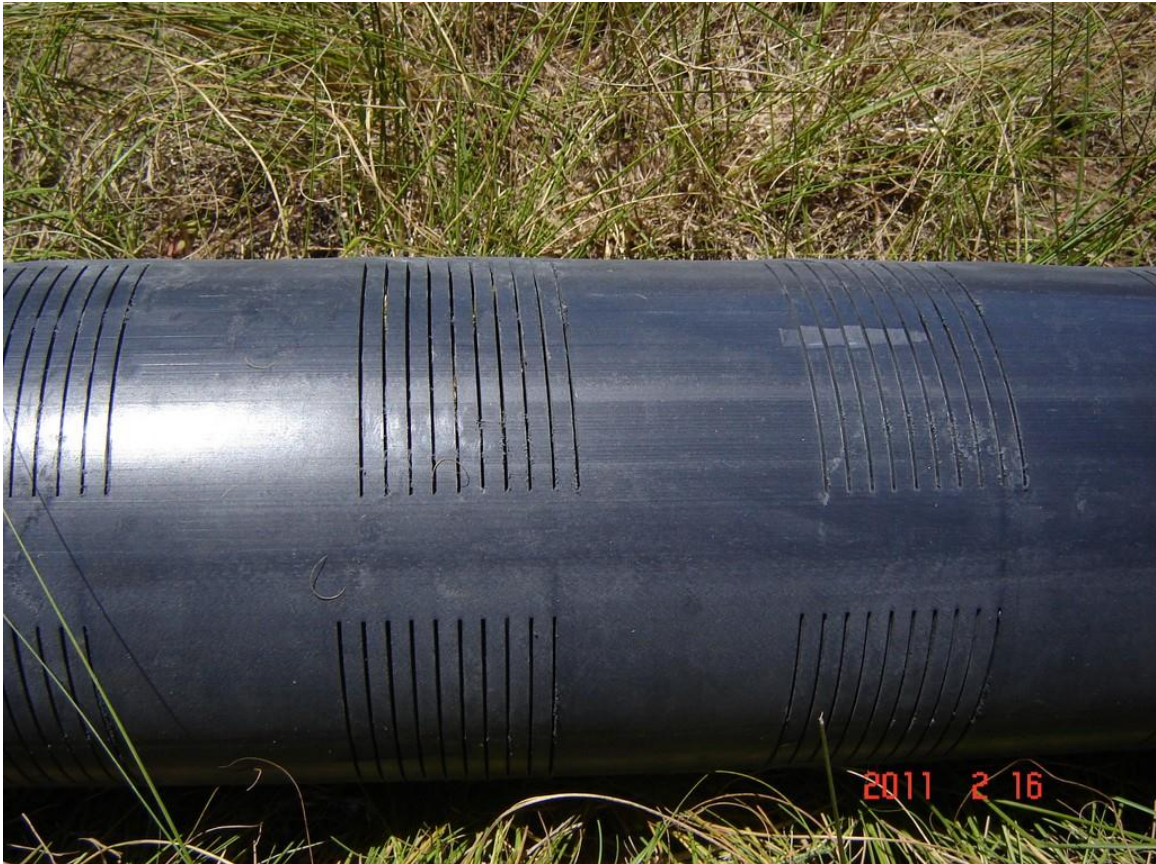
Figure 36: Slotted PVC casing.
