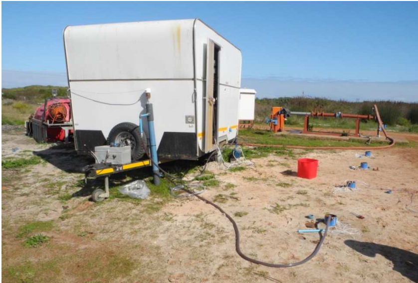
Figure 70: The modified experimental set-up for the ISIR at the study site after the first injection tests
