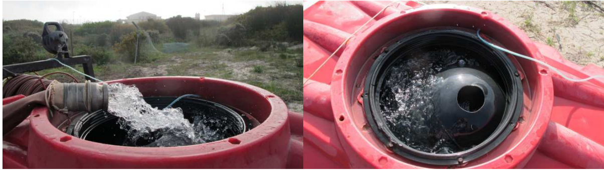
Figure 64: The abstracted groundwater was aerated by increasing the exposure to the atmosphere by splashing the water as it entered the tank (left) and recirculation within the tank(right)
