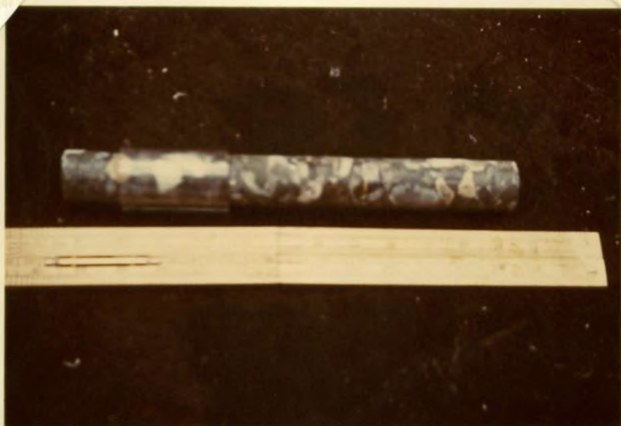
Plate V. -- Method applied in the determination of pebble sizes on a borehole core.
