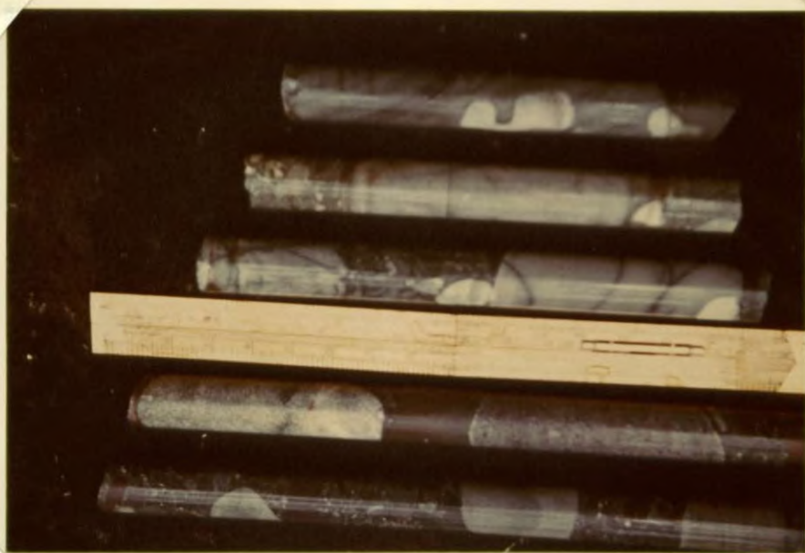
Plate VI. -- Specimens of borehole core with large pebbles showing cuts parallel to the apparent c-axis.
