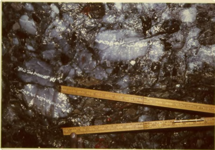
Plate VII. - Large pebbles of milky quartz orientated with their long axes parallel to the bedding-plane.
