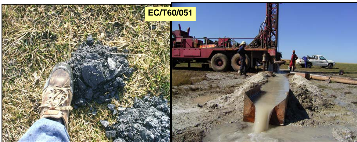
Figure 6.1.1a: Photos showing yield measurement and drilling residue - (Nel 2005, Lusikisiki Groundwater Feasibility Study)
