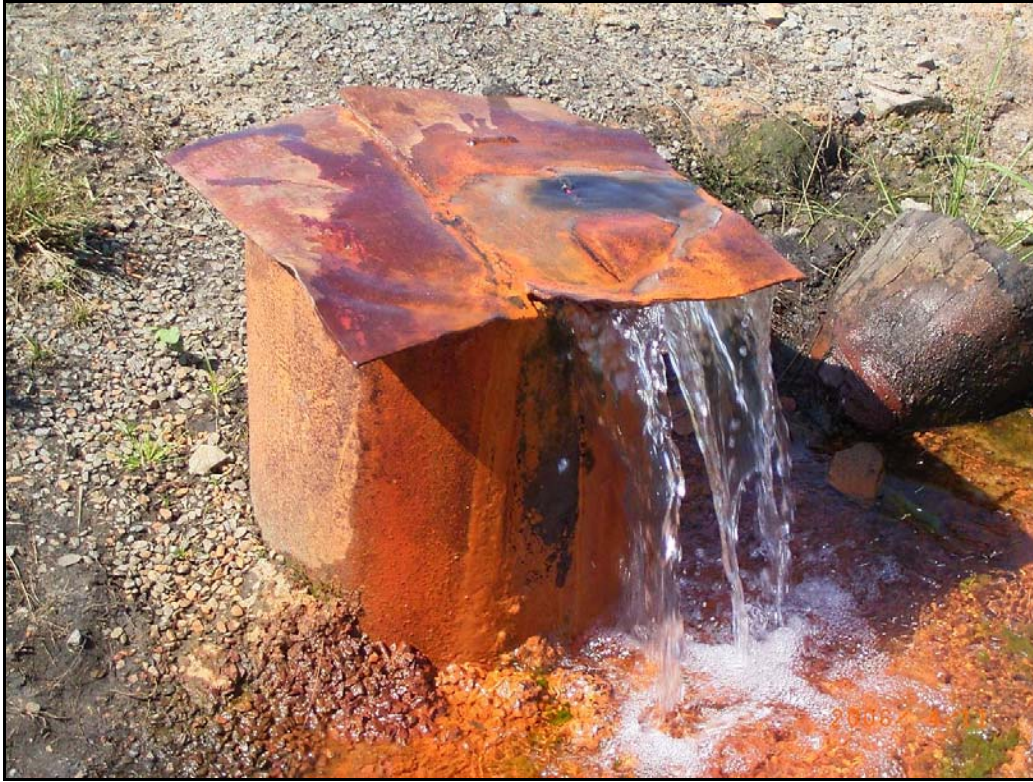
Figure 6.2.1b: Photo showing oxidation around EC/T60/054 - (Nel 2005, Lusikisiki Groundwater Feasibility Study)
