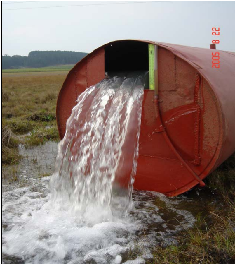
Figure 6.2.1: Borehole EC/T60/054 measured with U-Notch - (Nel 2005, Lusikisiki Groundwater Feasibility Study)
