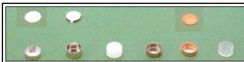
Figure 3.27: DSC sample pans 206
