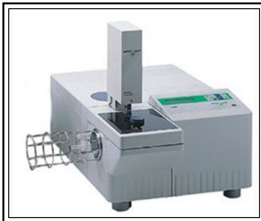
Figure 3.23: View of a TGA apparatus 202
