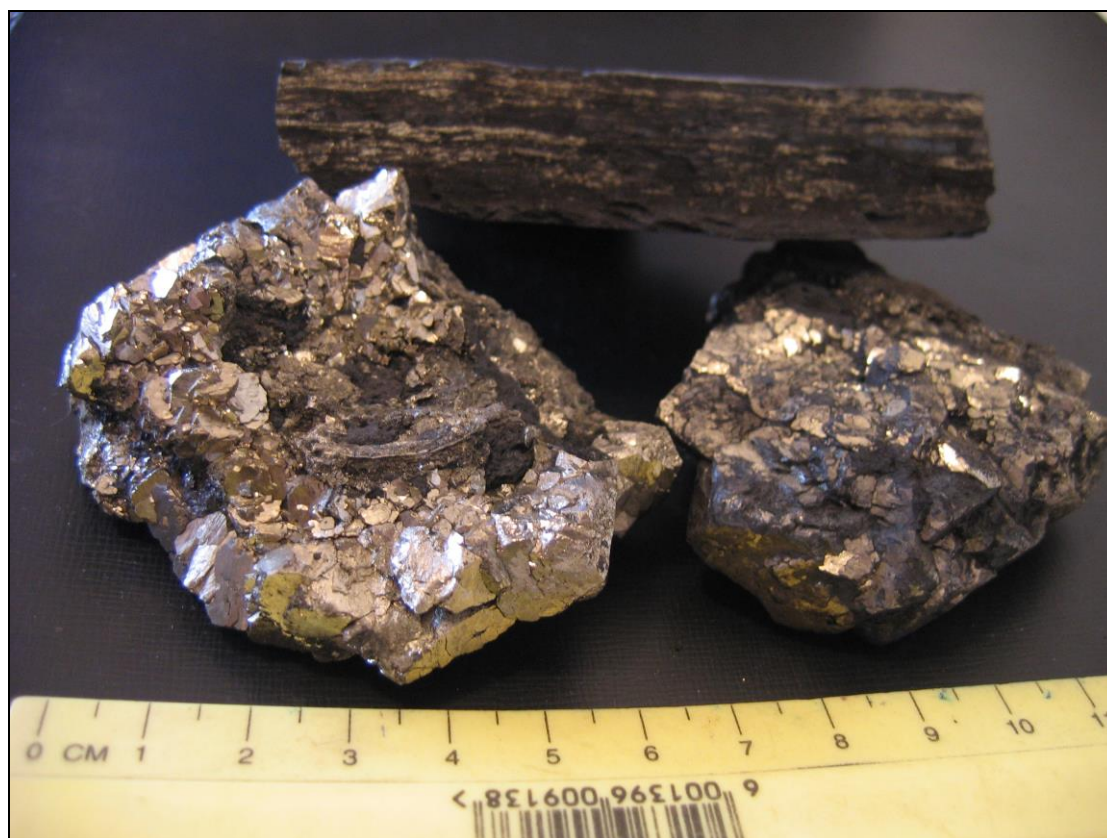
Figure 2.6.1(C). Massive and disseminated euhedral pyrite from the Leeuwpan Colliery, eastern Witbank Coalfield 1 .
