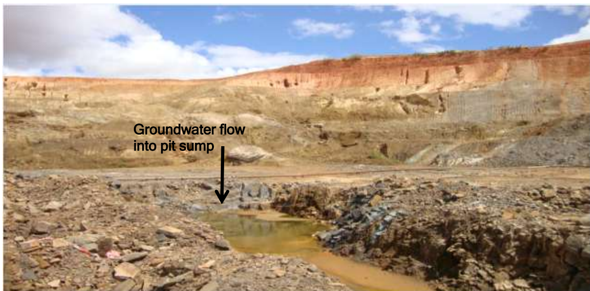
Figure 1-3: Groundwater flow into Pit 1 sump at Ruashi Mine
