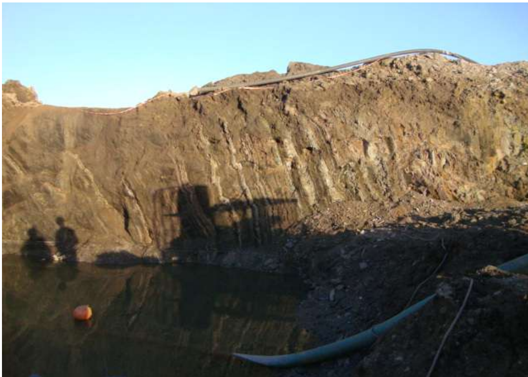
Figure 7-3: Black Ore Mineralised Zone showing weak and strong bands in Pit 1. The foreground shows ponding of groundwater adjacent to pit wall
