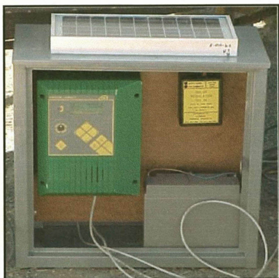
Figure 2.7: Data logger and power supply
