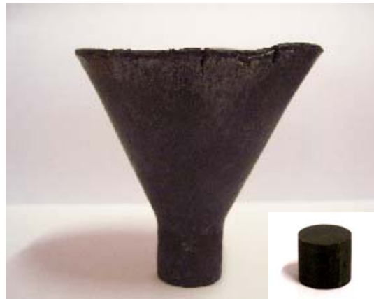
Figure 5.2: Molybdenum liner used, with sample extracted from the liner using spark erosion. Images do not have the same scale.
