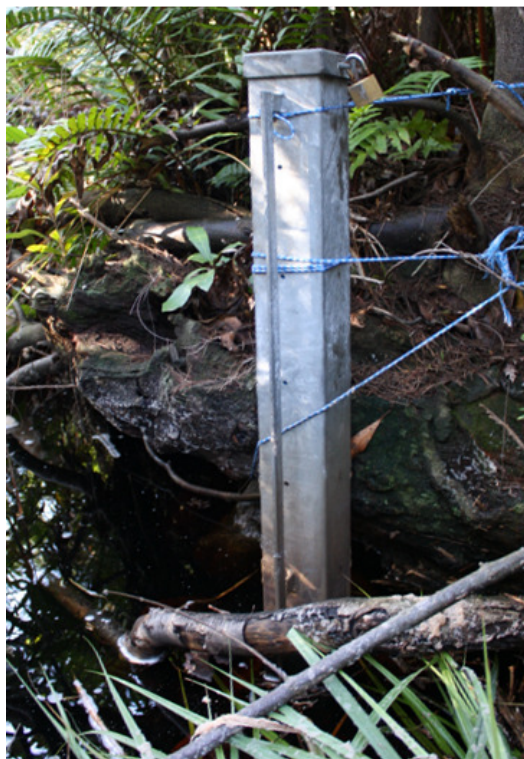
Figure 82. River 1 stilling well located in the Oudebosch River that flows down the middle of the valley.
