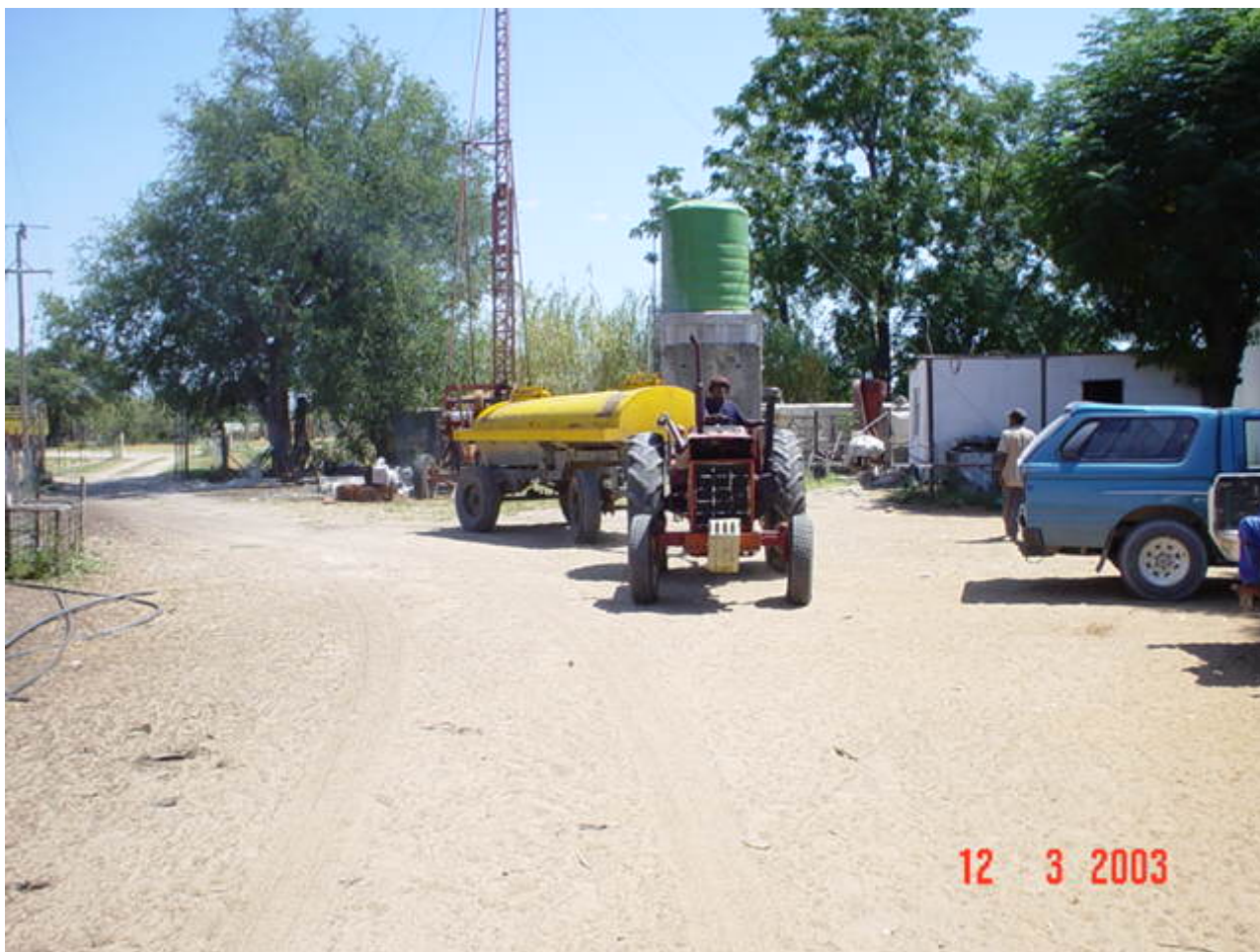
Plate 4. Carting of water and re-drilling of a dried up borehole on the farm Quarreefontein after the water level declined an estimated 60 m due to proximate irrigation abstraction.
