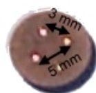
Figure 3.7: A photograph of a Cu sample holder with four 1 mm depth holes drilled into it. The specific separation distances are indicated on the photograph.
