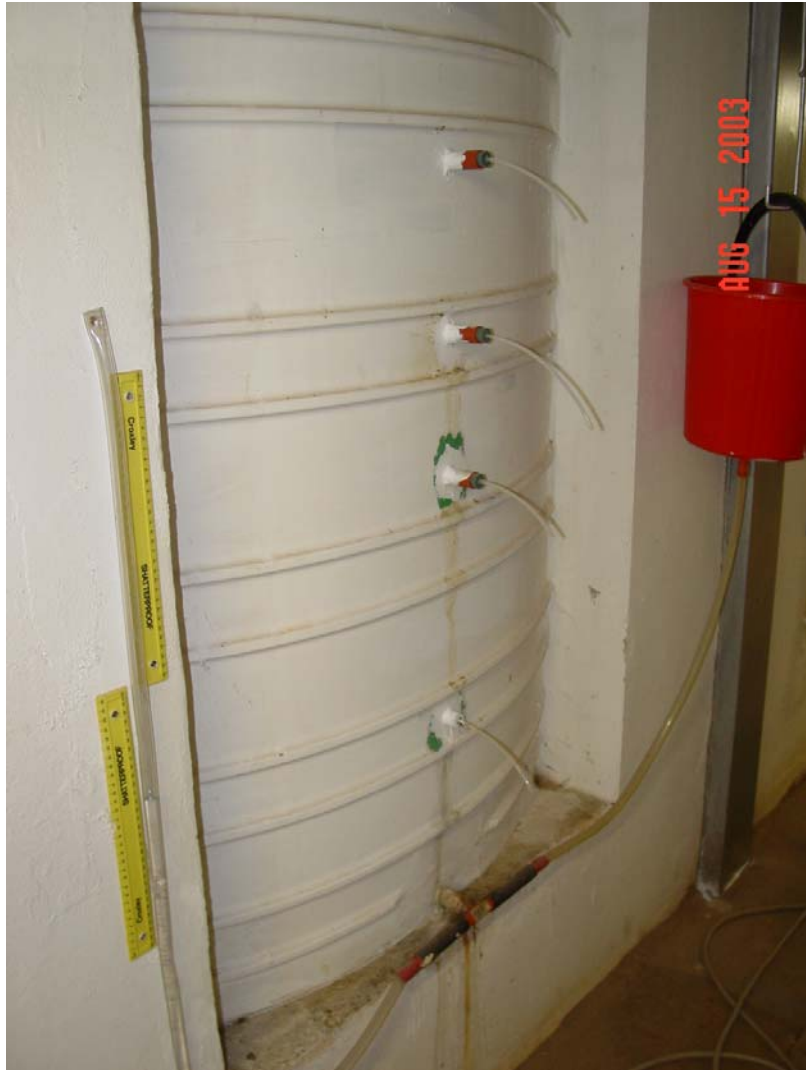
Plate 4.1 Ceramic cups installed from the access chamber side of the lysimeters at different depths from the soil surface.
